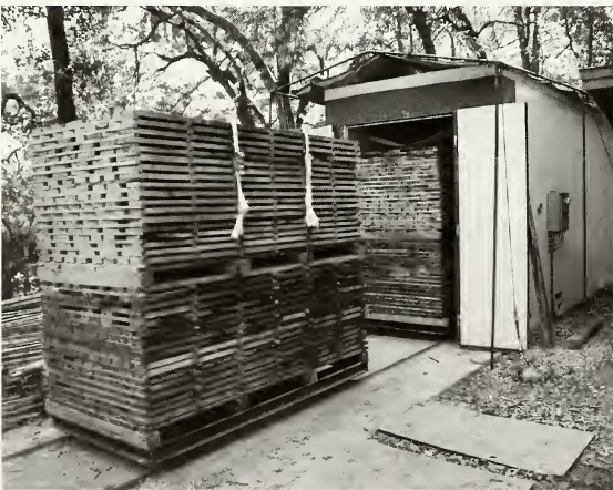
FIG. 3. Tanoak lumber stacked and ready for loading into a low-temperature, forced-convection, lumber dry kiln at a small mill operation in Santa Cruz Co., California.
